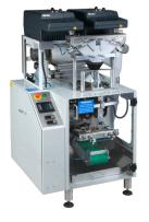
The SC-9100H2 unit with twin counting heads and escrow system produces up to 80 sachets per minute.
