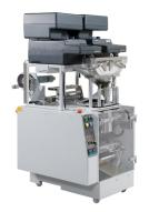
SC-9100H2 with coin fed to both counting head from a SCAN COIN bulk coin lift.
